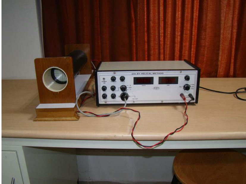
Figure 1: Apparatus for the charge to mass ratio experiment.
