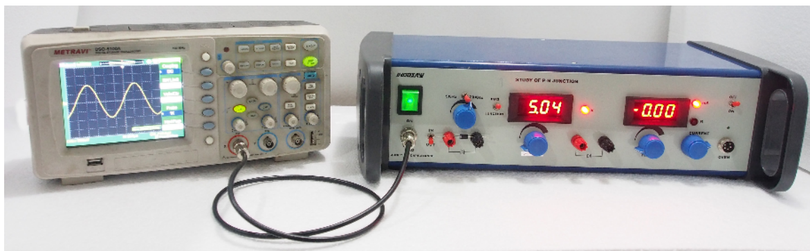
Fig. 8 : Experimental Arrangement to Determine Depletion Capacitance of Sample IN5402
