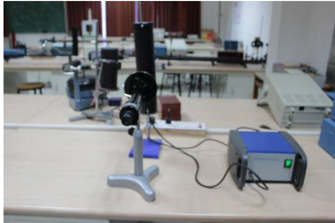
Figure 6.1: Experimental setup for the polarimeter.
