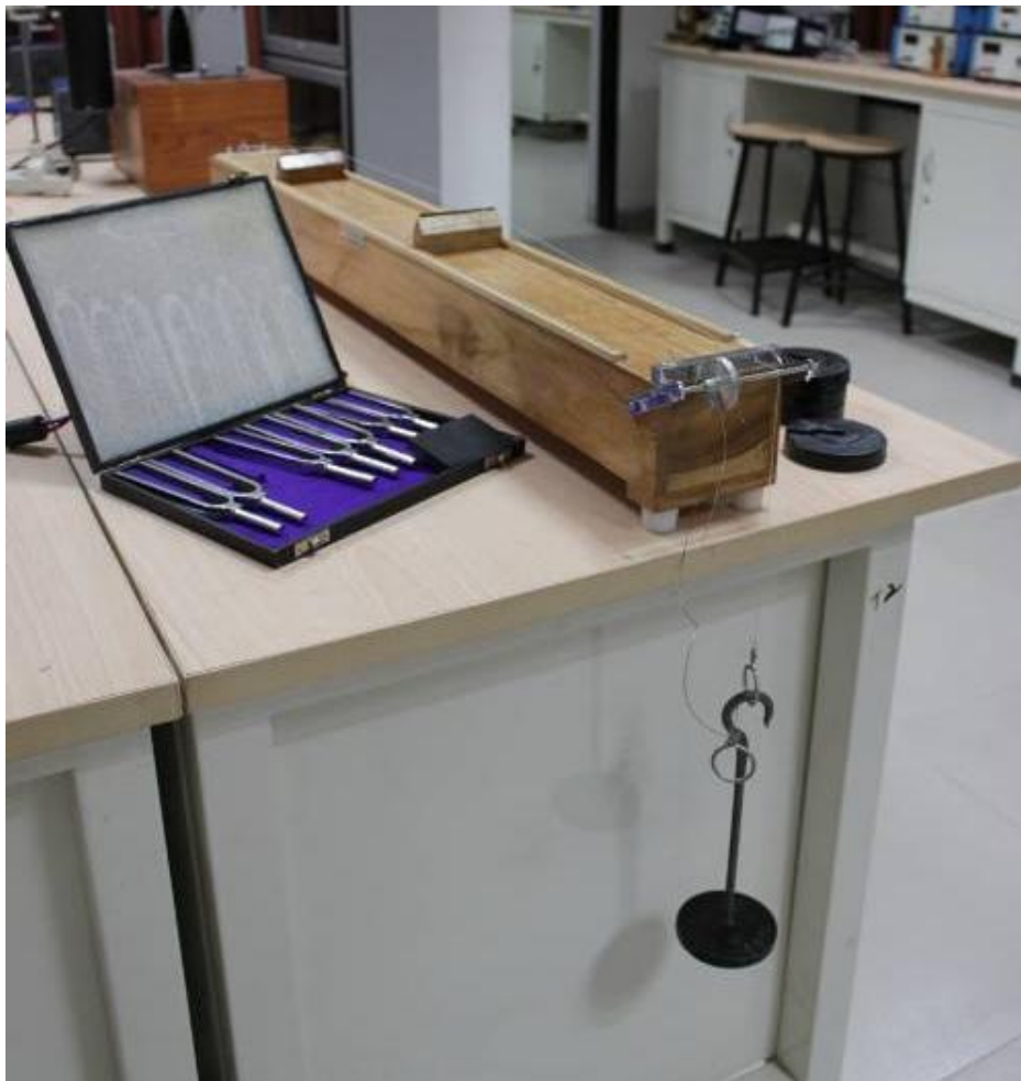
Figure 1.1: Experimental setup for sonometer.
