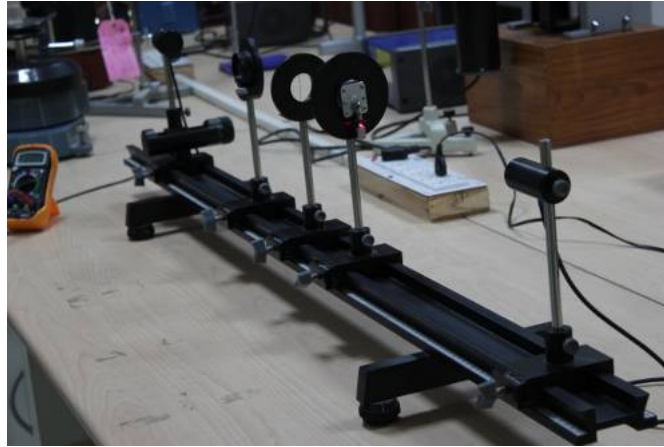
Figure 9.1: Experimental setup for single slit diffraction showing the optical bench and mountings.
