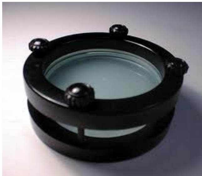
Figure 8.4: Glass plate and plano-convex lens arrangement.
