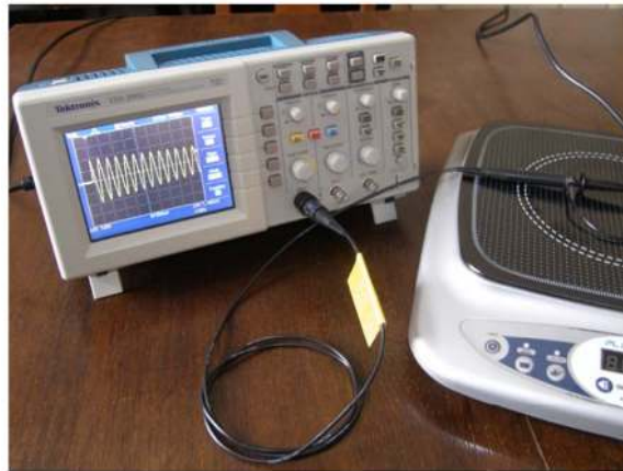
Figure 10.3: Induction cooker connected to an oscilloscope.
