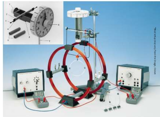
Figure 4.2: Experimental set-up for determining the torque due to a magnetic moment in the magnetic field.
