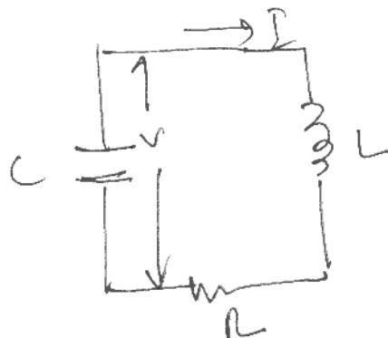
$V$  is +ve if upper capacitor plate is truly charged. +ve current direction defined by the arrow. Then,
