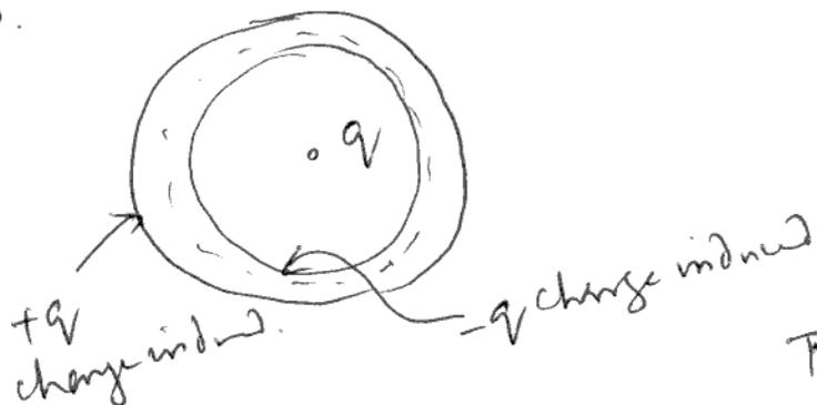
Consider Gaussian surface that encloses charge  $q$  & the inner surface of the conducting shell.
