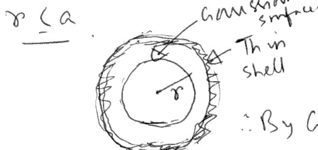
Charge enclosed by Gaussian surface = 0. Since all charge resides on the surface of shell.
