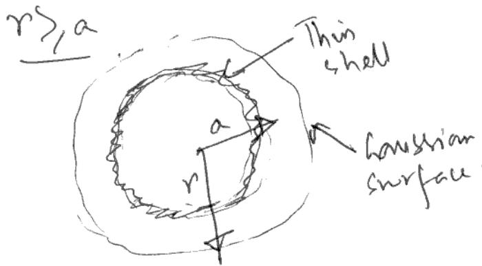
Charge enclosed by Gaussian surface =  $Q$ .
