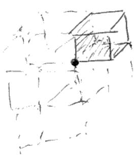
When you shift the charge to a corner, try to construct a bigger cube with twice the edge length, such that the charge is at the center of this bigger cube. The bigger cube will be made of 8 small ones.
