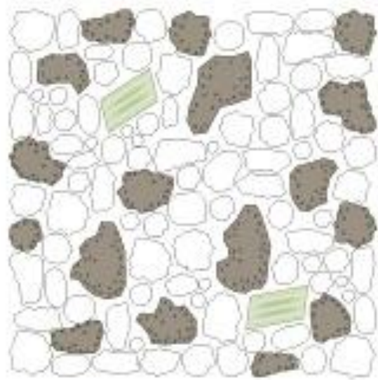
(c) Lithic sandstone: rock-fragment-rich
