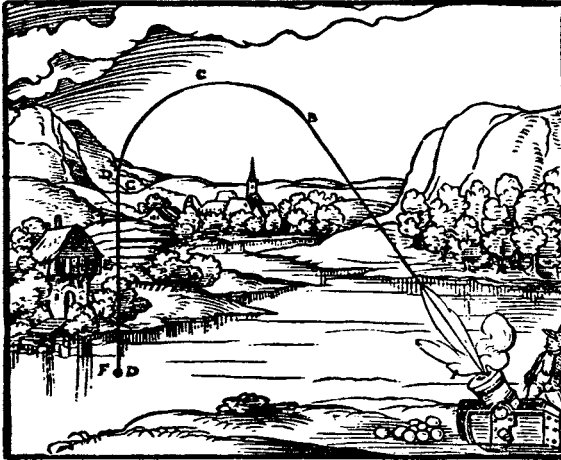
Figure 10.1. An Aristotelian representation of a cannonball's trajectory. It illustrates the Aristotelian concept that the trajectory consists essentially of two separate motions, unnatural (away from the ground) and natural (toward the ground). In this figure the transition between unnatural and natural motions is a circular arc. (From G. Rivius, Architectur, Mathematicchen, Kunst , 1547).
